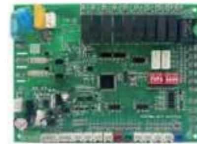
单系统 SINGLE COMPRESSOR CONTROL
